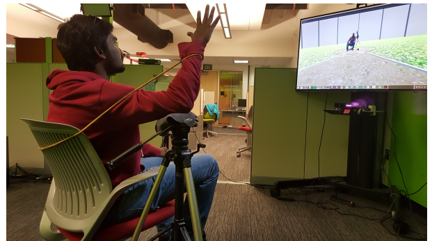
Figure 12: Experimental setup showing a person playing ShotPut game with his right arm tied up with bungee cord to simulate patient condition.
